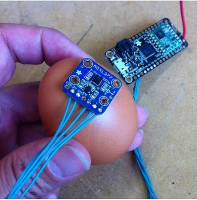
OMSI performed tests with an accelerometer and found that an egg cracks as it decelerates at more than 60 g or 60 times the normal gravitational force. Some type of cushion is needed to protect the egg during its deceleration phase on impact to keep it below 60 g.
